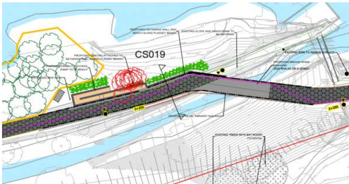
Figure 3-105: Proposed plan of ramp and Bridge 5 at Plassey Beach
